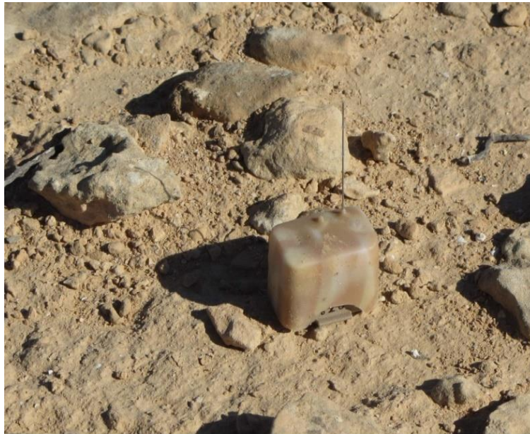
Figure 1.10. A camouflaged acoustic sensor [15]
