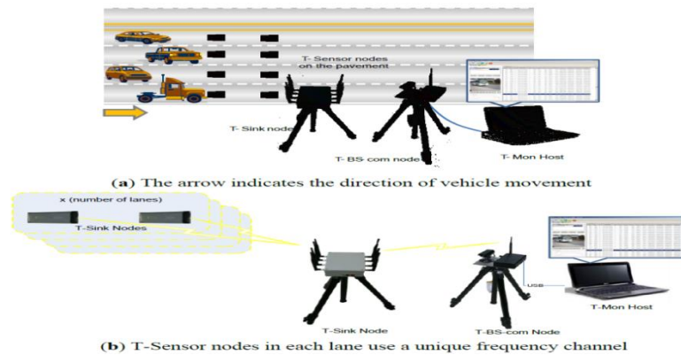
Figure 1.55. A complete representation of the WSN based Transportation monitoring system [58]
