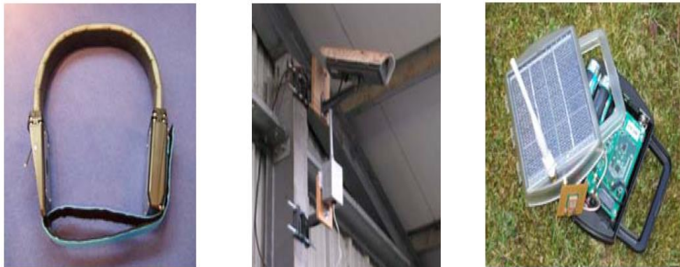
Figure 1.32. a) An antenna diversity collar, b) deployed BS and c) a solar powered antenna diversity router. [37]
