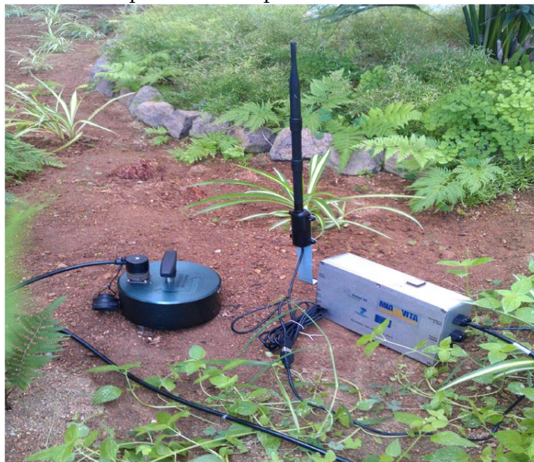
Figure 1.22. A depiction of a geophone sensor with a wireless antenna deployed in the field [26].
