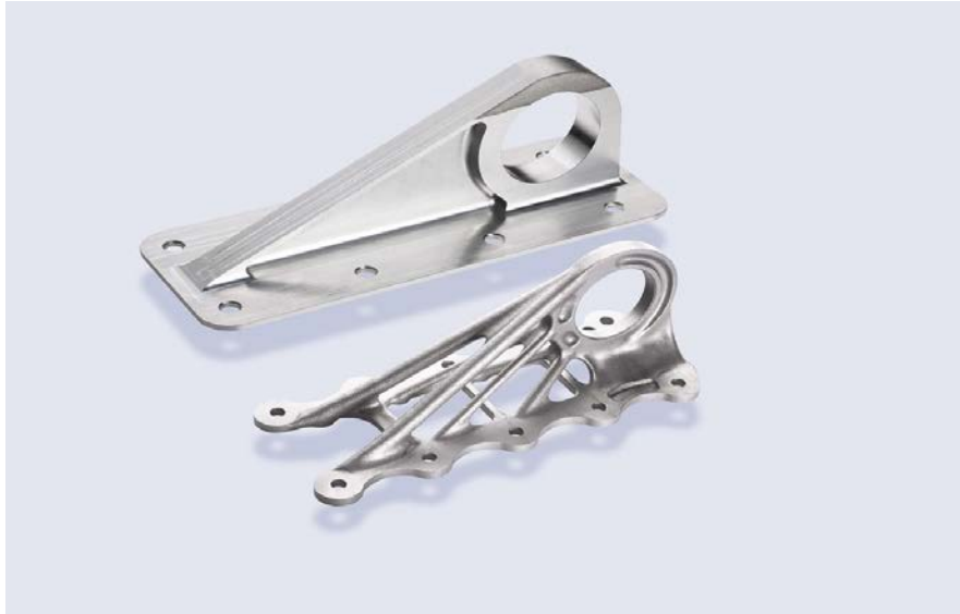
Figure 4 3D-printed components of an Airbus Jet (3D-Printed 'Bionic' Parts Could Revolutionize Aerospace Design, 2017)
