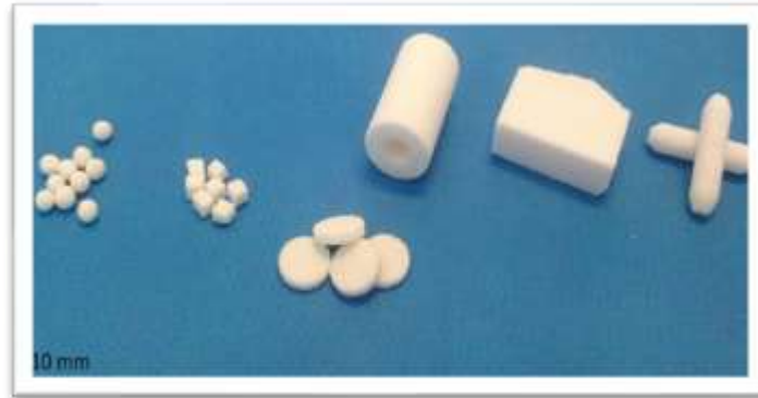
Image 4-7: Coral implants of various shapes and sizes for bone tissue engineering applications. Adapted from: (Manassero et al., 2016)
