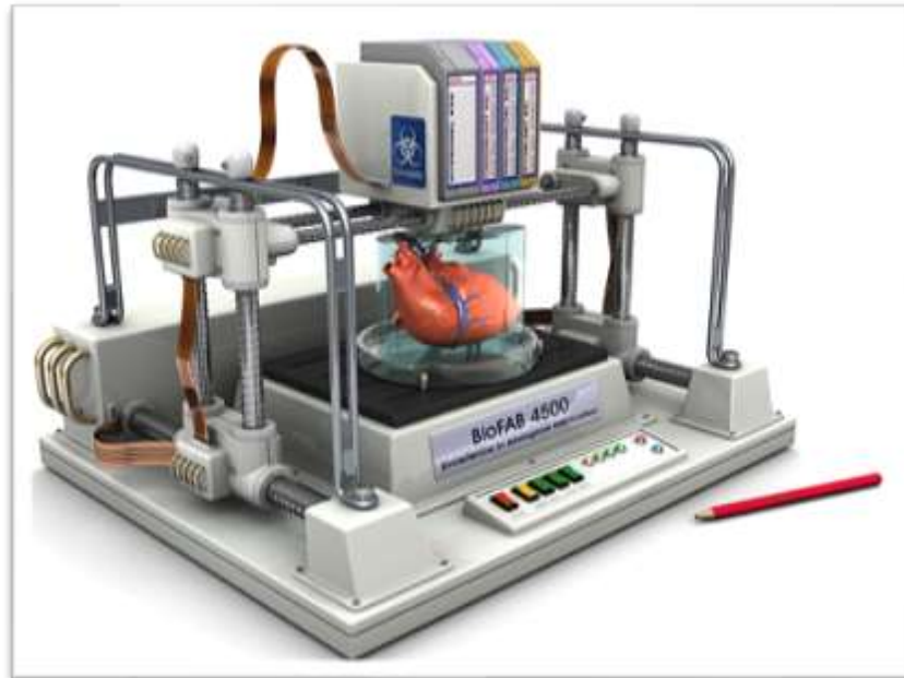
Image 5-42: Organ printing concept system: 3D functional tissues and organ are printed on-demand. Adapted from: (Ozbolat & Yu, 2013)
