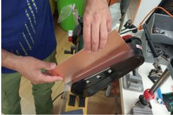
Figure 36. Cutting the FR4 board.
