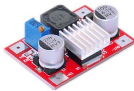
Εικόνα 3.20 - DC-DC Boost Converter 2A 5-56V (cableworks, High Voltage DC-DC Boost Converter 2A 5-56V, n.d.)
