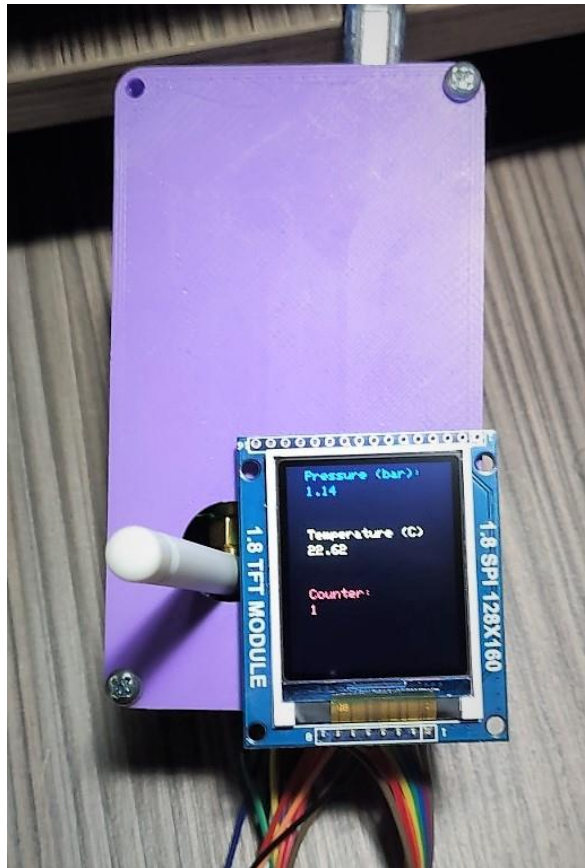
Figure 11 - 1.8" TFT Module Application Example
