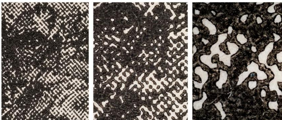
Letterpress halftone reproduction with an earlier dot structure seen at 10x, 30x, and 50x magnification.
