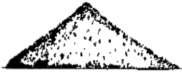
Figure F.3— Aggregate saturated surface-dried; almost complete collapse but definite peak still visible and slopes are angular
