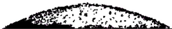
Figure F.4 — Aggregate nearly oven dry; no distinct peak, surface outline close to being curvilinear
