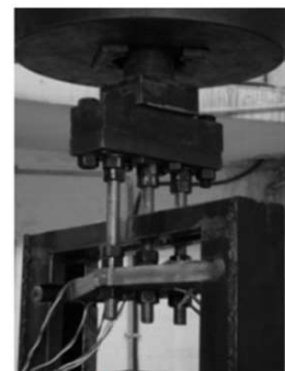
Fig. 4. Testing layout of rhombic steel plate dampers
