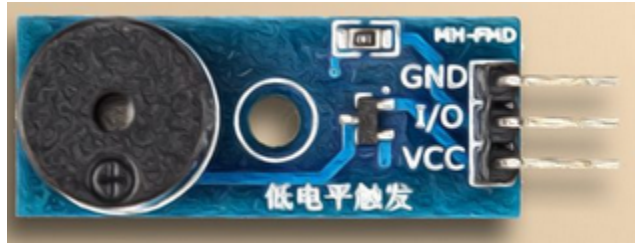
Εικόνα 2.24: Buzzer module ( https://electropeak.com/learn/interfacing-active-buzzer-with-arduino/ )
