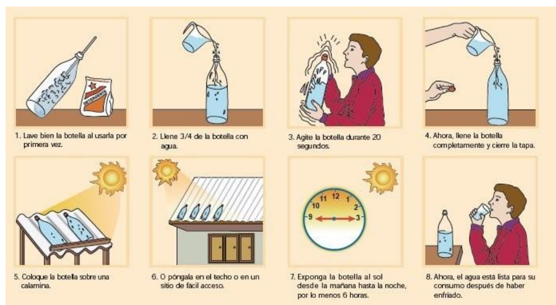
Image 6. Steps to carry out solar disinfection – SODIS (Ecoinventos.com)
