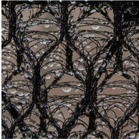
Image 6 Fog nets, Clous fisher (Floating springs, Harvesting drinking water with fog nets, n.d.)
