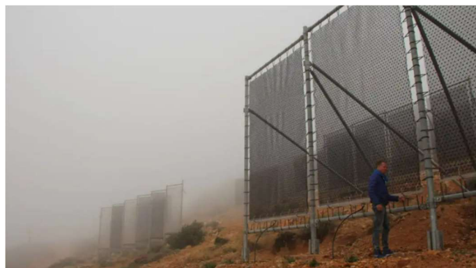
Image 3 Cloud fisher, fog nets (Floating springs, Harvesting drinking water with fog nets, n.d.)
