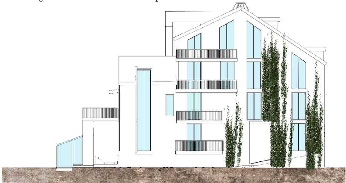
Image 69 Schematic diagram of the window improvement on the north façade (Source: by Author)
