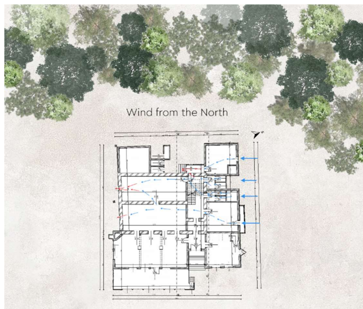
Image 64 The wind entering the building (ground floor) from the north (Source: by Author)
