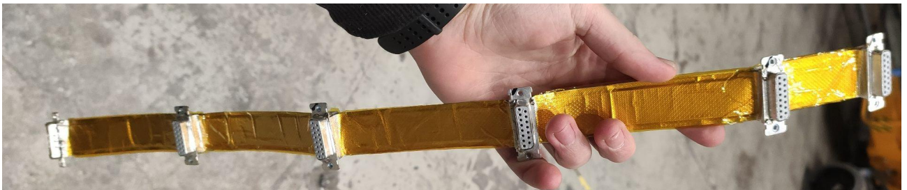
Figure 5.14: The refurbished branch controller flat cable.
