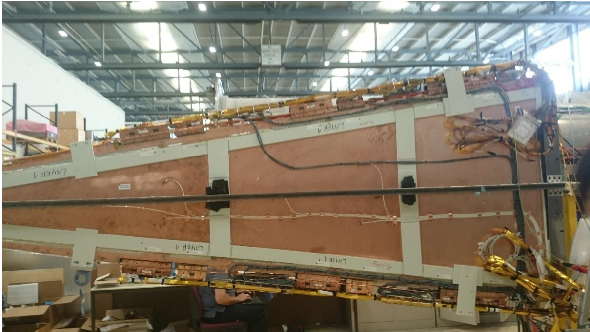
Figure 74: A small sTGC wedge with all electronics installed.
