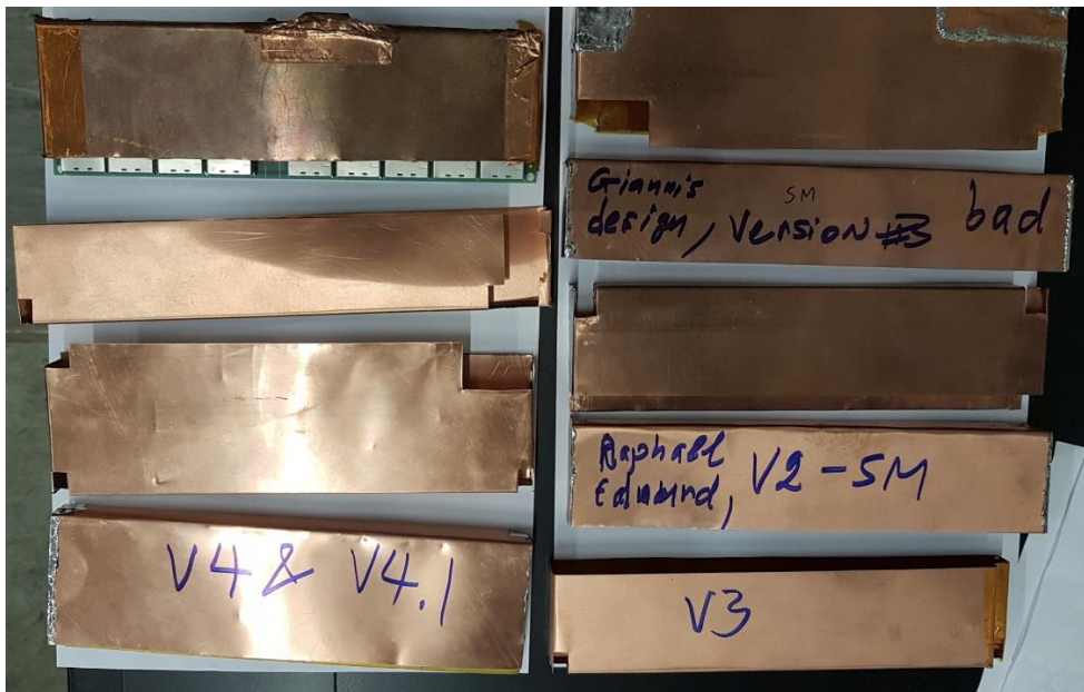
Figure 50: Some of the Faraday cages prototypes. The one marked as V3 is the final design.
