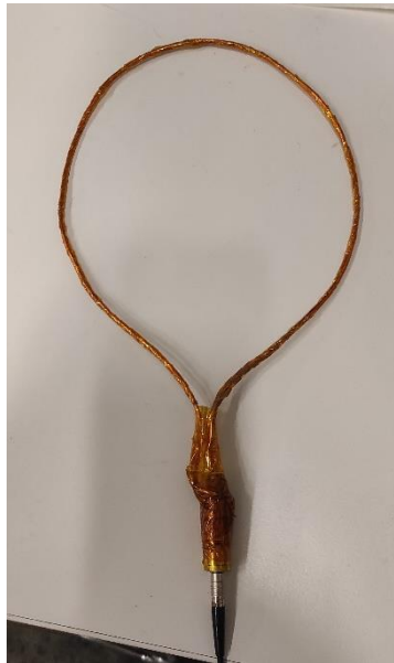
Figure 56: The magnetic loop antenna used in the noise investigation. The antenna is wrapped in Kapton tape and has a BNC connector for being connected to the oscilloscope.
