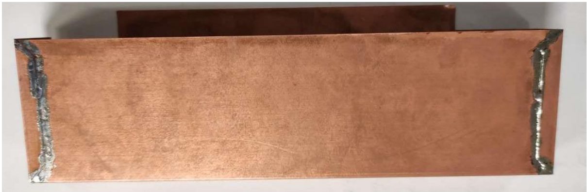
Figure 77: ADDC Faraday cage manufactured by a company and soldered manually.
