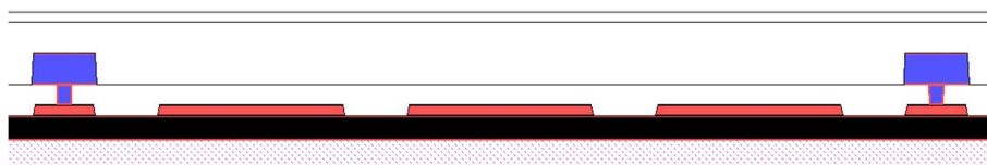
Figure 30: Cross-section of serpentine structure 1kohm resistor.
