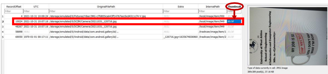
Figure 66. Parsing “imagecache0.sqlite” (tool used: DB Browser for SQLite, Examined Device: LG G6).
