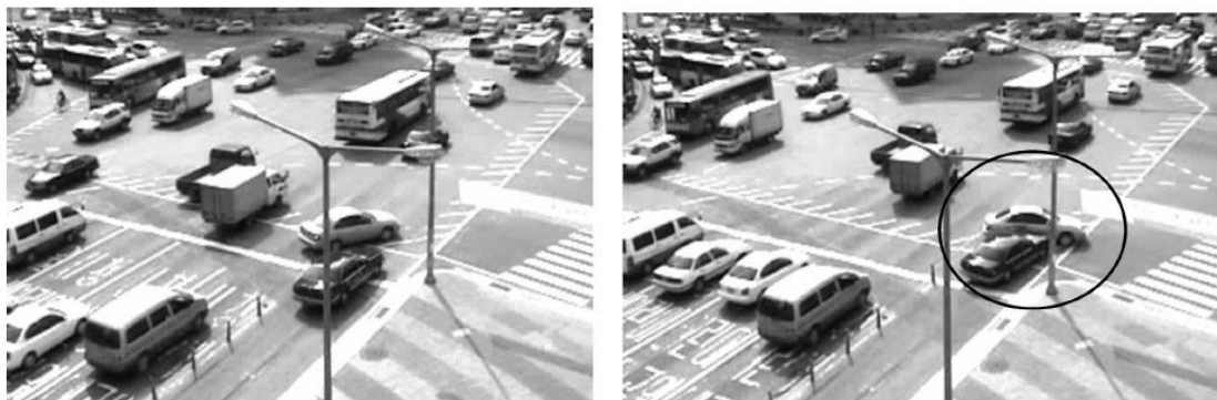
Figure 1.10: Images from a traffic control camera before (left) and after (right) automatic accident detection [9]
