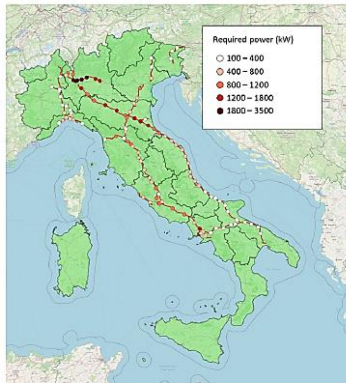
FIGURE 7: Power to be installed to meet the changing needs of EVs on the SAs belonging to ASPI network expected in 2030.
