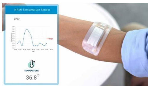
Figure 1.80: Flexible Patch for Temperature Monitoring through the IoT, developed by NAMI [144].
