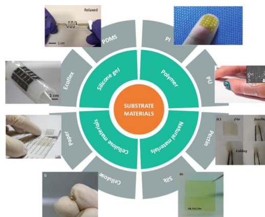
Figure 1.22: A visual classification of the flexible substrates used in flexible biomedical sensors [32].
