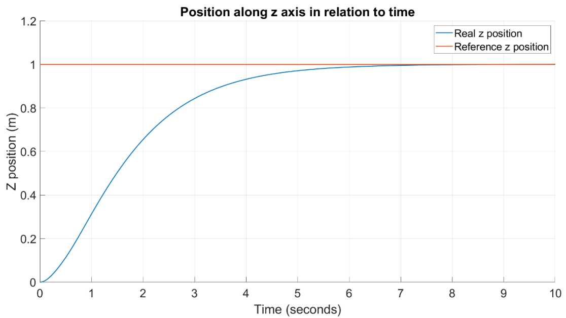
Figure 13. Position z in relation to time for step reference input equal to -1[m] using the PID design
