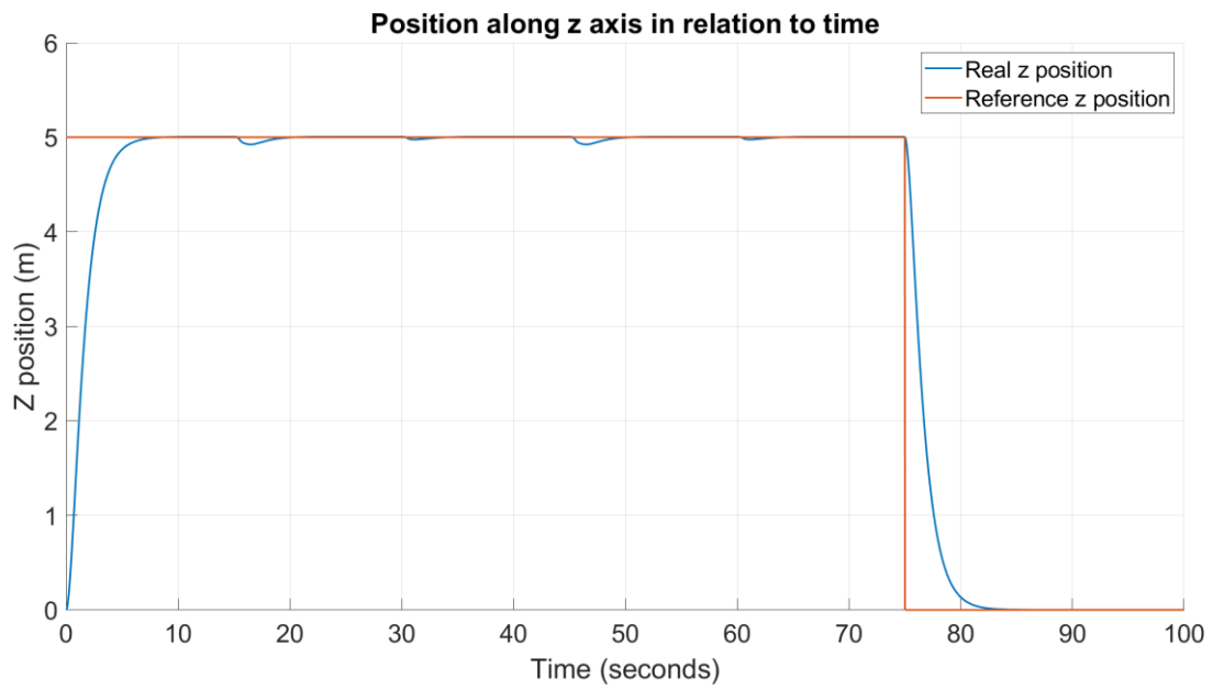
Figure 24. Position z (altitude) in relation to time for step path reference using the PID design
