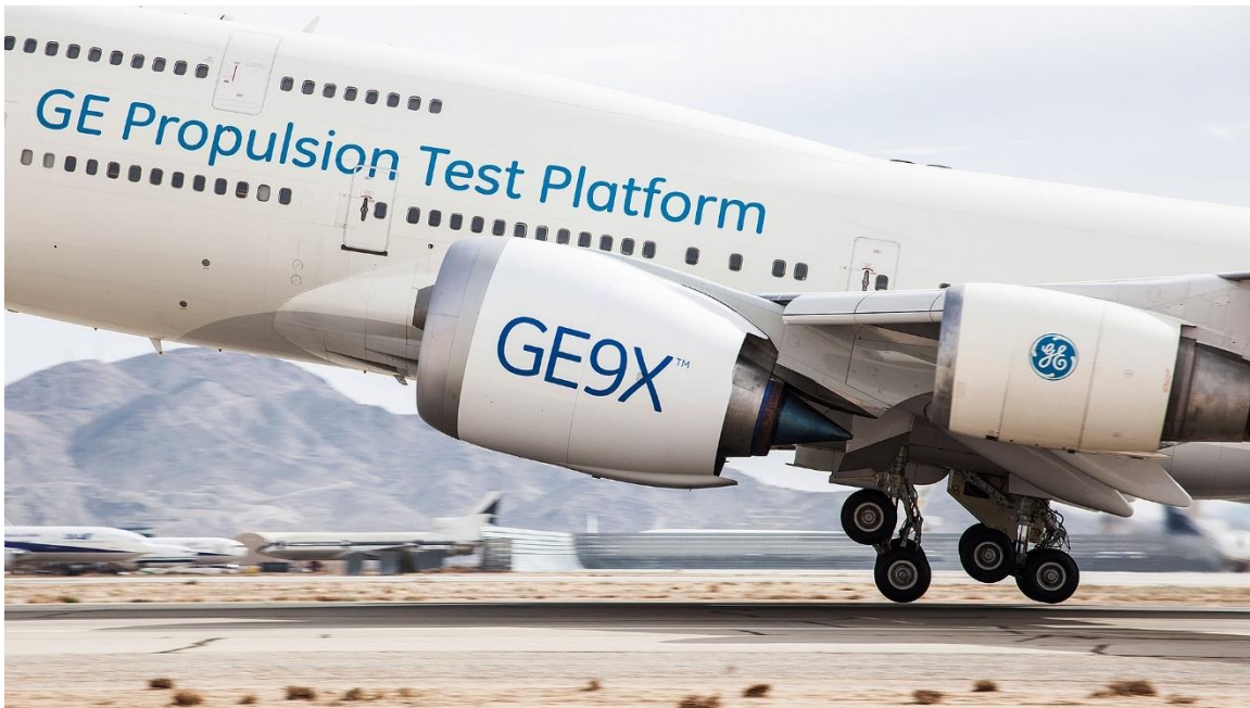
Figure 2.2: The GE9X, the world's most powerful aircraft engine yet, mounted on General Electric's 747 test platform. The GE9X was exclusively developed to power Boeing's latest aircraft, the Boeing 777X [9].
