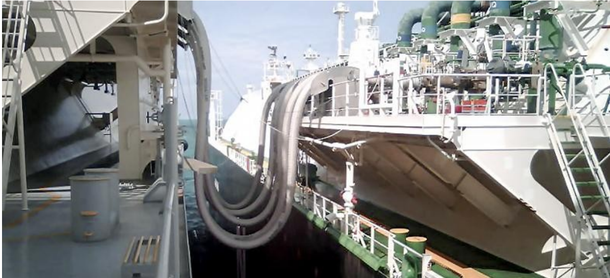
Picture 5: LNG transfer from carrier to FSRU [7]
