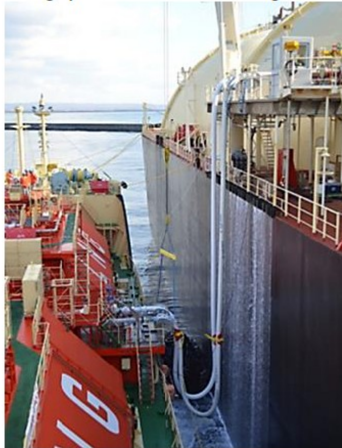
Picture 15: Water curtain during STS transfer [32] Wärtsilä, 2014
