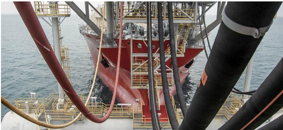
Picture 6: Continuous regasification process on FSRU and sending high-pressure NG to the shore [7]
