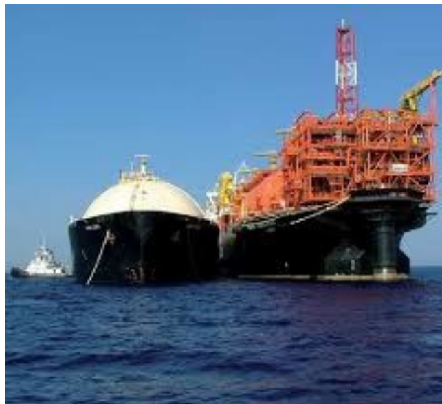
Picture 14: LNG transfer side by side through loading arms [31]
