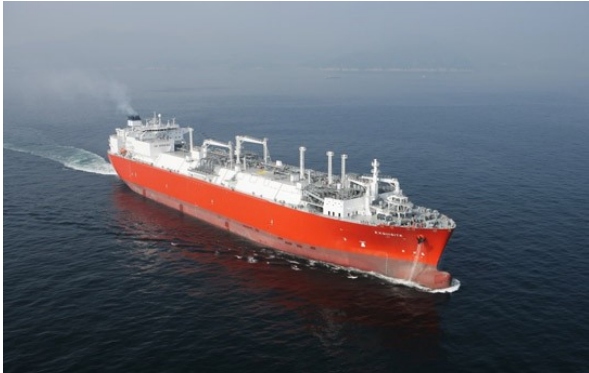
Picture 1: Membrane Tanks with regasification facilities on the deck Source: Courtesy Excelerate
