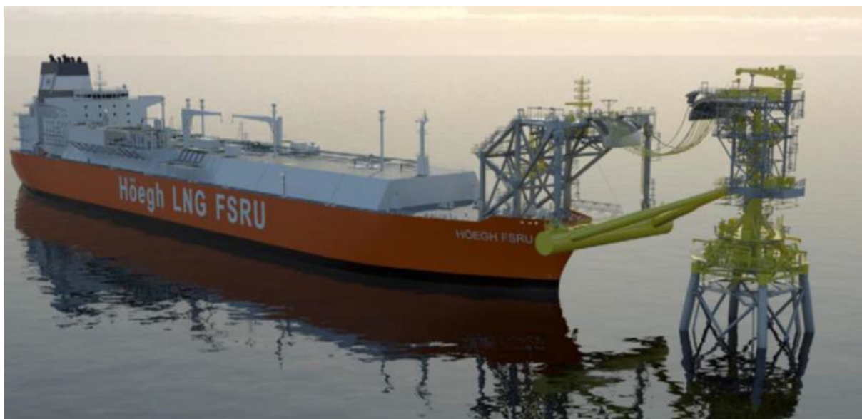
Picture 7: Tower Yoke Mooring System [19]
