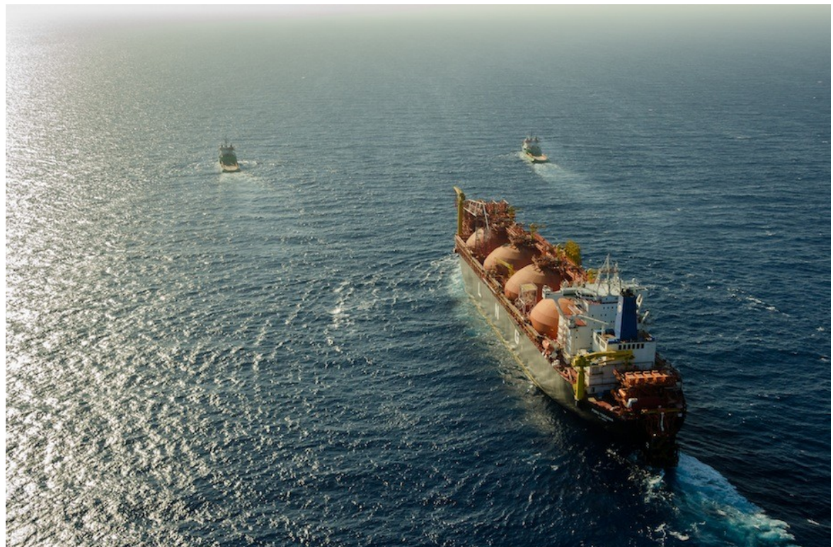
Picture 2: FSRU Toscana with Moss type tanks [18]
