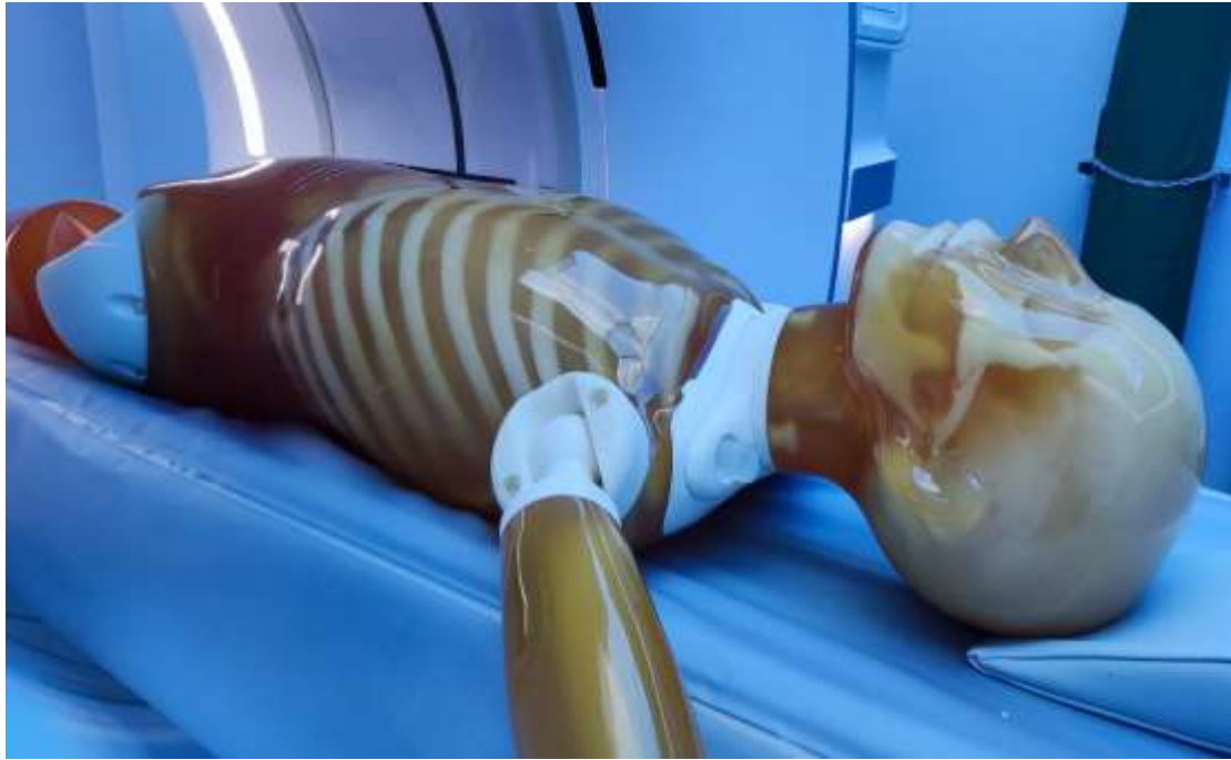
Figure 11: PBU-60 Whole body phantom as placed for the Chest/Abdomen/Pelvis irradiation with the arms raised as in actual patient positioning. Picture from personal archive.
