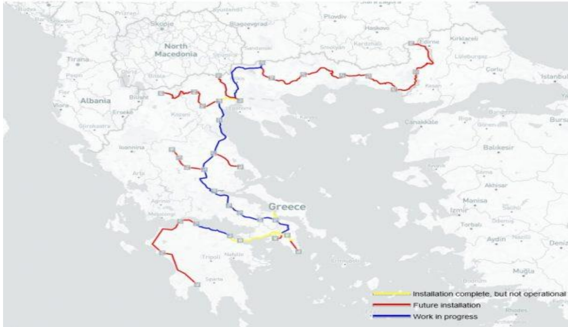
Installation of the European Train Control System in Greece
