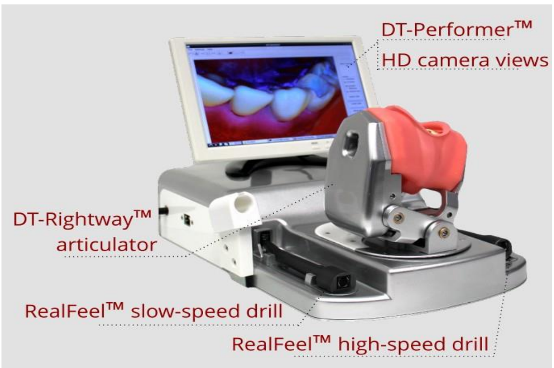
Σχήμα 16: DenTeach comprises the DT-Instructor (instructor workstation) and DT-Student (student workstation) that communicate through a cloud-based communication channel.
