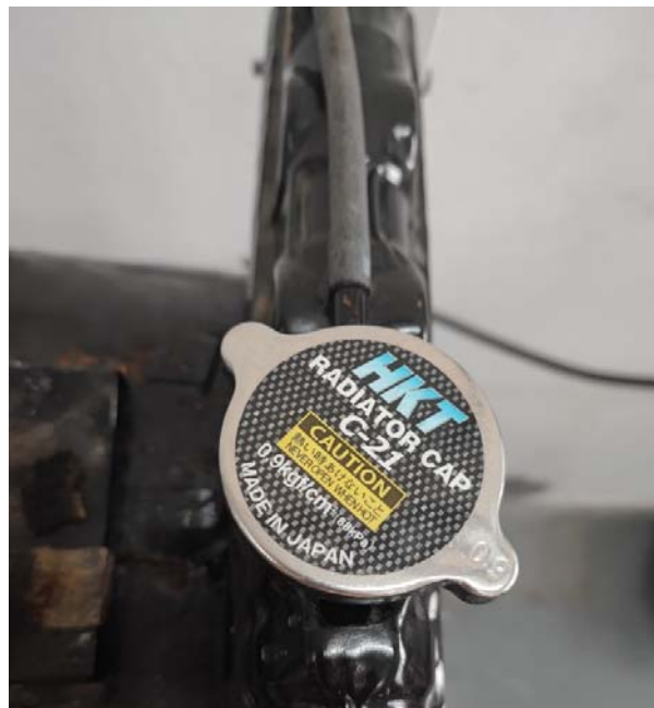
Figure 34: Radiator Cap and Overflow Pipe
