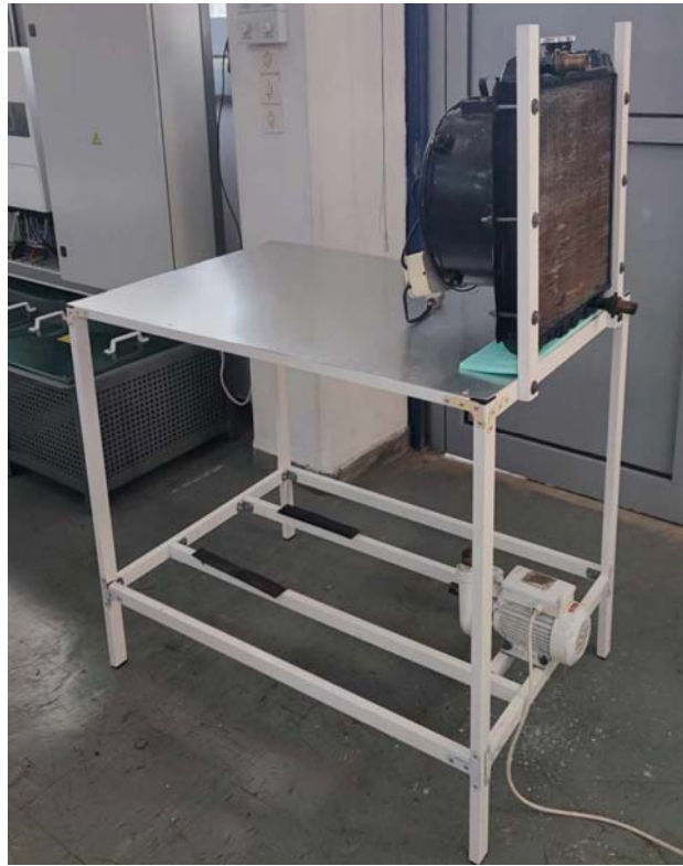
Figure 78: Heat Exchanger Secured with brackets on Workbench
