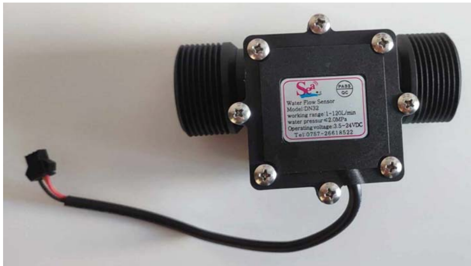
Figure 43: Water Flow Sensor
