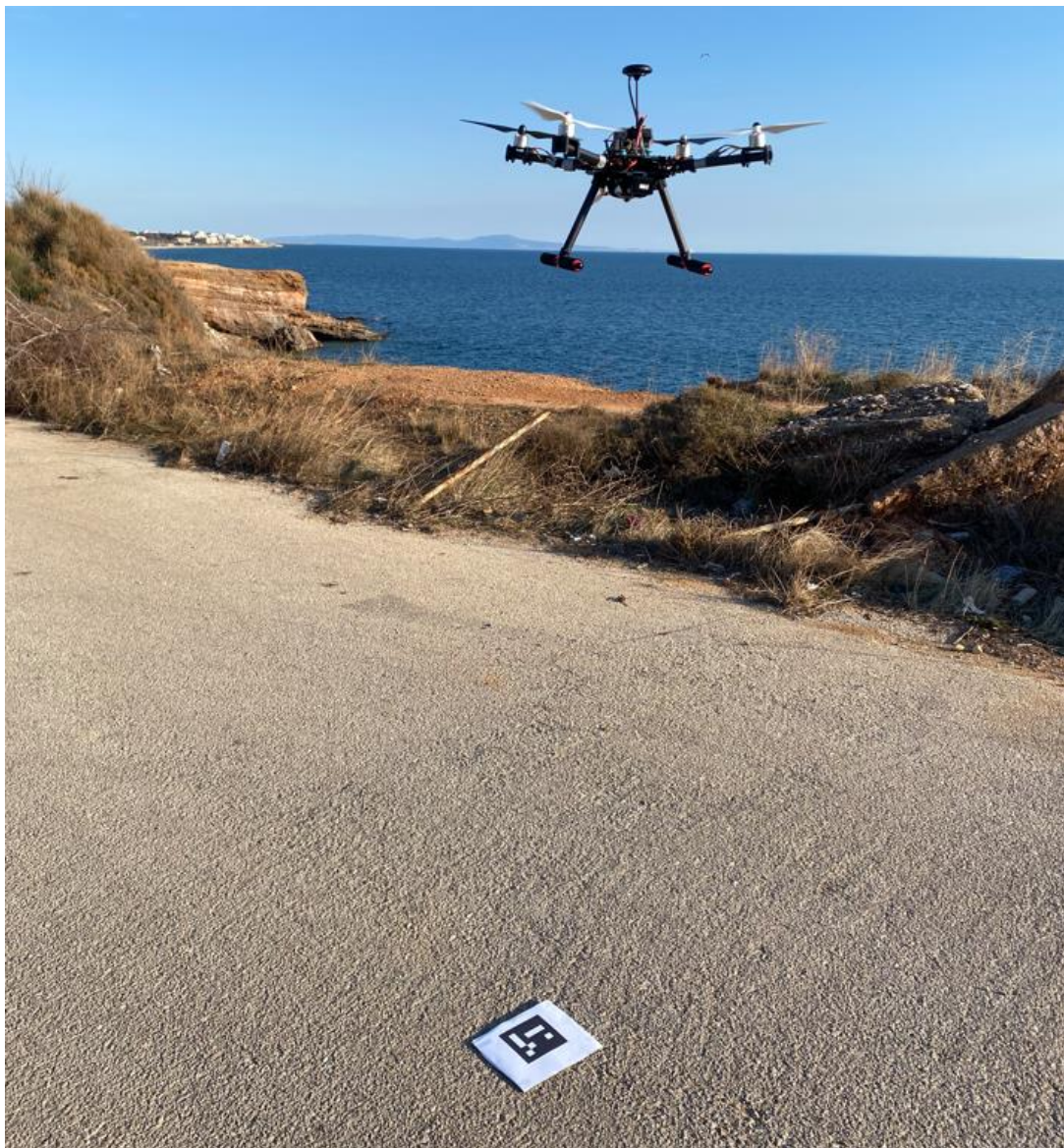
Εικόνα 43 Preparing for landing using aruco marker and openCV
