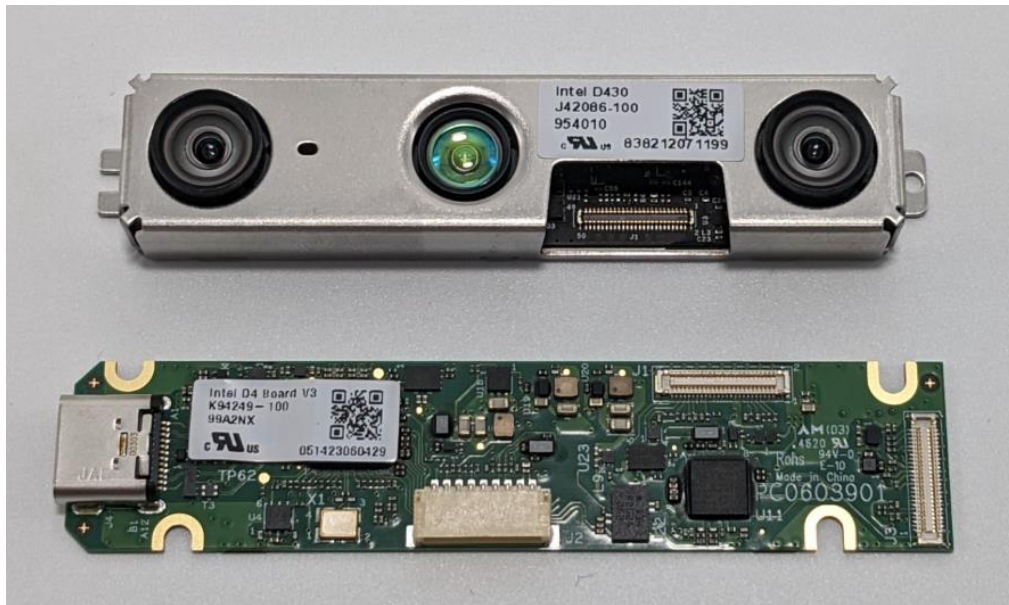
Figure 6: Main components of D435 RealSense 10
