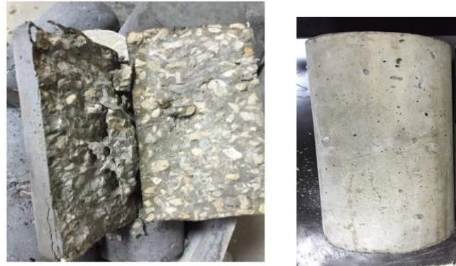
Fig. 14. Non-Rubberized Concrete Cylinders Splitting into Two Halves. Fig. 15. Rubberized Concrete Cylinders without Splitting After Failure.
