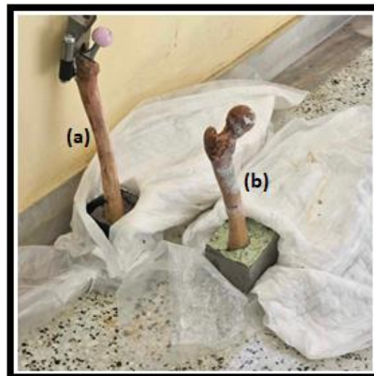
Figure 95: Cadaveric specimens used for the experimental procedure. (a) is the left and implanted femur, and (b) is the right intact femur.
