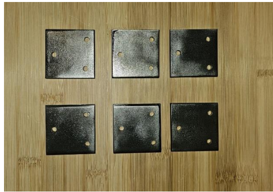
Figure 105: The special square tiles that can be used to adjust the position of (4) at the vertical axis.
