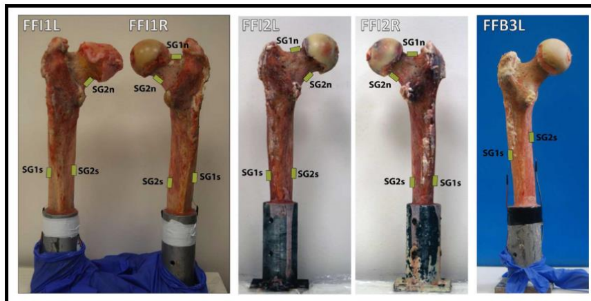
Figure 18: The five femurs embedded in a steel cylinder and the strain gauges' locations on the femurs [42].
