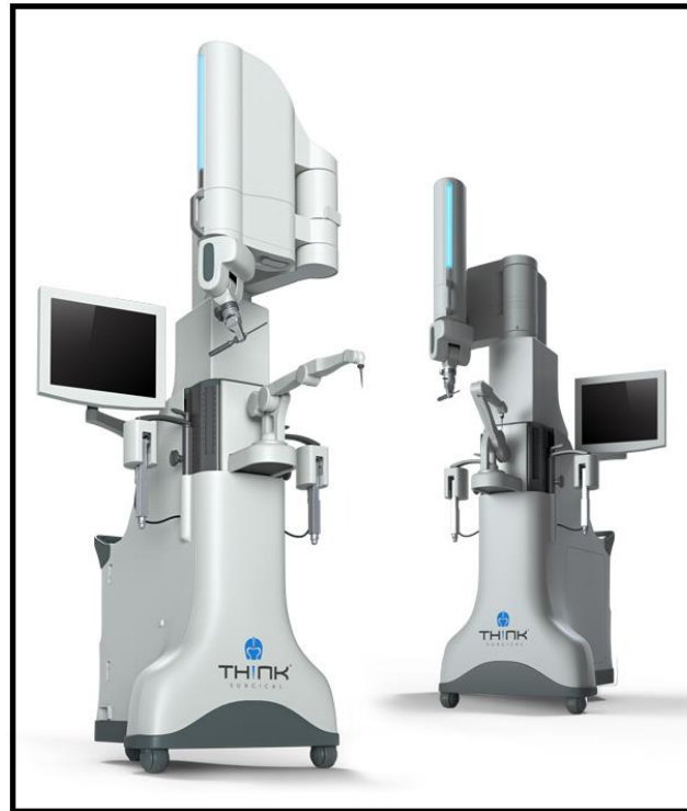
Figure 15: TSolution One, a fully-active robotic system [35].
