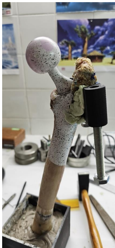
Figure 119: This figure presents the damage at the great trochanter done by the excessive temperature that was developed by the polymerization of the PMMA.
