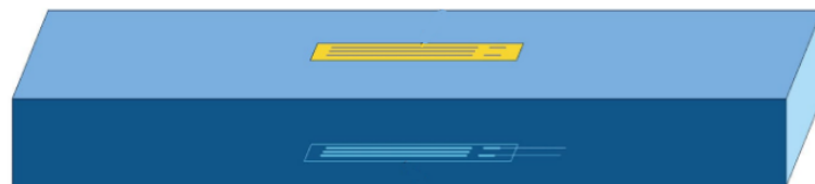
Figure 69: Placing the two active strain gauges on two opposite sites for the bending half-bridge configuration [85] (edited).
