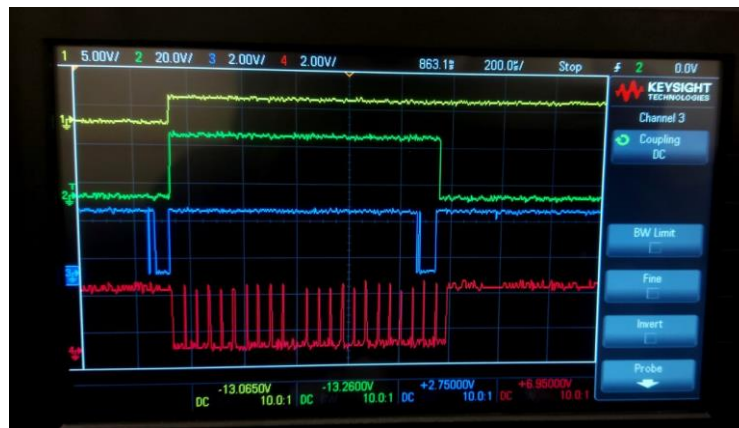
Figure 30: Serial communication signals zoomed
