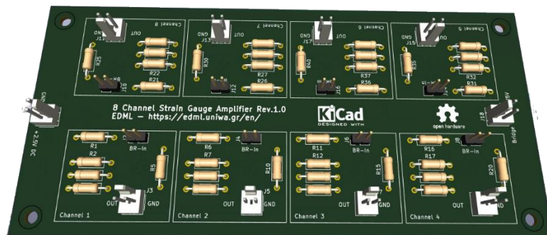
Figure 12: 8-Channel Strain Gauge Amplifier Top View (KiCad 3D view)
