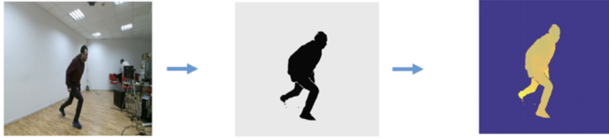
Figure E.3: Depth map based on skeleton representation: Using depth pixels in previous 2d estimation, find the corresponding 3d voxels based on 3d skeleton data).
