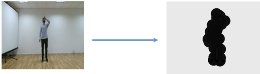
Figure E.1: Human silhouette: Map 3D joint coordinates to 2D space. Estimate human silhouette based on skeleton data.
