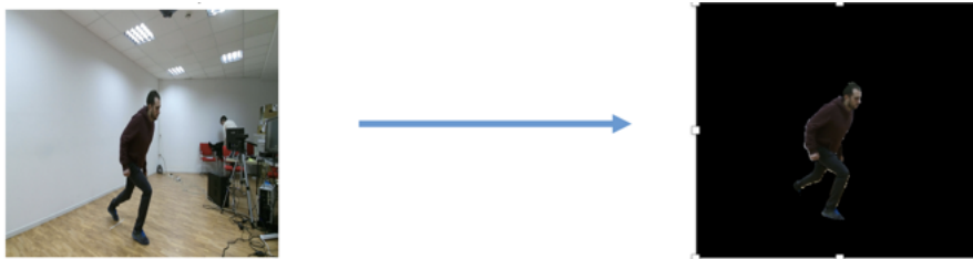
Figure E.2: RGB information: Map Depth to RGB pixels, and use their colour value to create RGB image in Depths' resolution. Remove background based on depth values around skeleton data.
