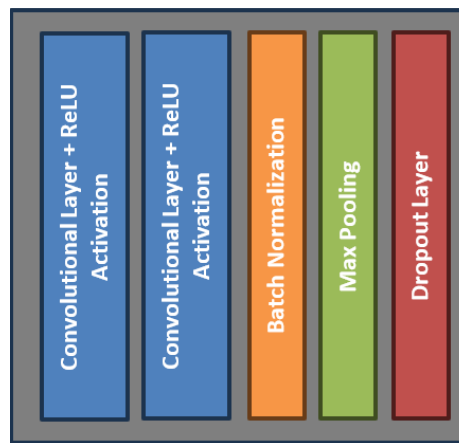
Figure 11: Convolutional Block of State Encoder
