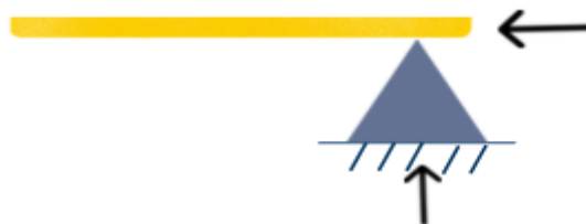
Εικόνα 21: Παράδειγμα άρθρωσης, PIGSO Learning: Types of supports & reactions ( https://pigsolearning.com/civil-engineering )
