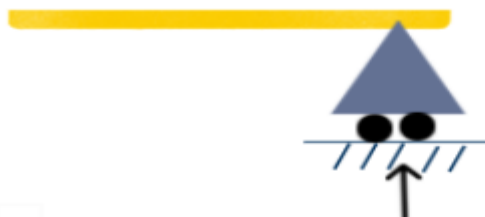
Εικόνα 20: Παράδειγμα κύλισης, PIGSO Learning: Types of supports & reactions ( https://pigsolearning.com/civil-engineering )
