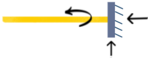
Εικόνα 19 Παράδειγμα πάκτωσης, PIGSO Learning: Types of supports & reactions ( https://pigsolearning.com/civil-engineering )
