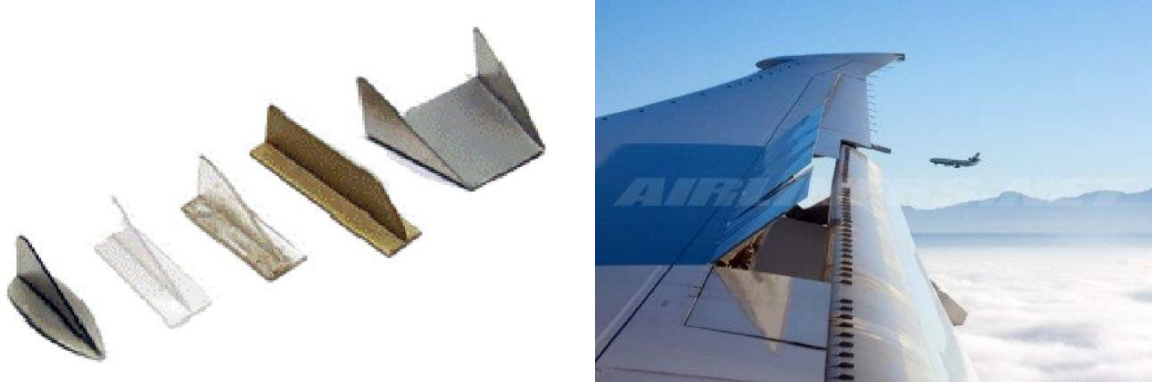
Figure 8 Left: Various types of vortex generators. Right: Installation of vortex generators on the flap. [22]
