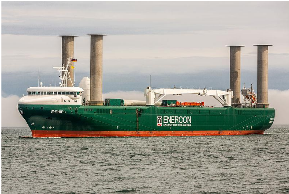
Figure 3 E-Ship 1 with Flettner rotors mounted [5]
