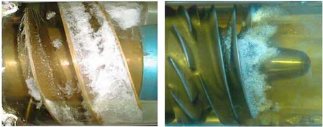
Picture 13 Cavitation in turbopump inducers. Here is shown the vaporization of the fluid that occurs on the vanes of the inducer during its operation [11]
