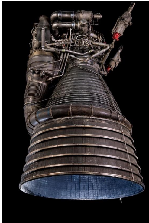
Picture 1: The F-1 engine, with 1.5 million pounds of thrust, was the powerplant for the first stage of the 363-foot long Saturn V launch vehicle that took astronauts to the Moon for six successful landing missions between 1969 and 1972 in the Project Apollo program [2].
