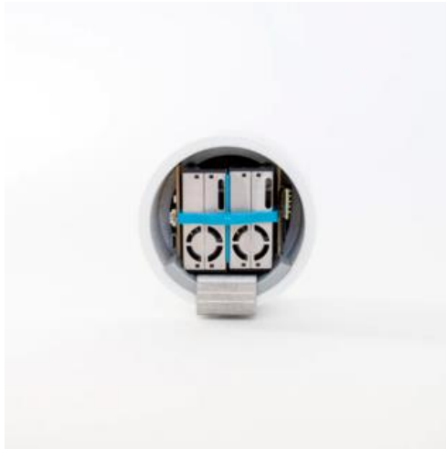
Σχήμα 4.2: PA – II – SD Air Quality Sensor. [35]
