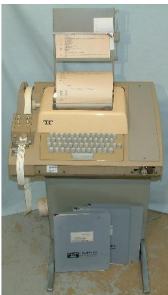
Figure 6, ASR Teletype machine used to interact with IBM mainframes. One of the first command line interfaces, displaying on a sheet of paper
