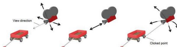
[Default camera navigation: (1) pan with left mouse button, (2) shift with mouse wheel, (3) rotate with right mouse button]
