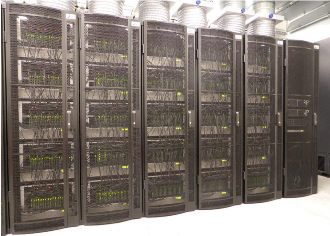
Σχήμα 4-5: 500 000-core SpiNNaker Human Brain Project platform
