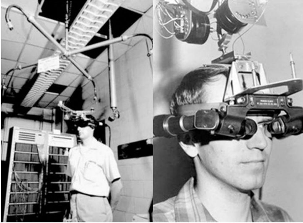
Image 2-3 Ivan Sutherland's first VR Head Mounted Display, "The Sword of Damocles",1968 (Paro, Bulsara, & Hersh, April 2022)
