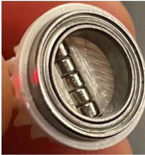
Image 5-7 Gear with the magnets and rolling bearing (LucidVR, Lucidglove, n.d.)
