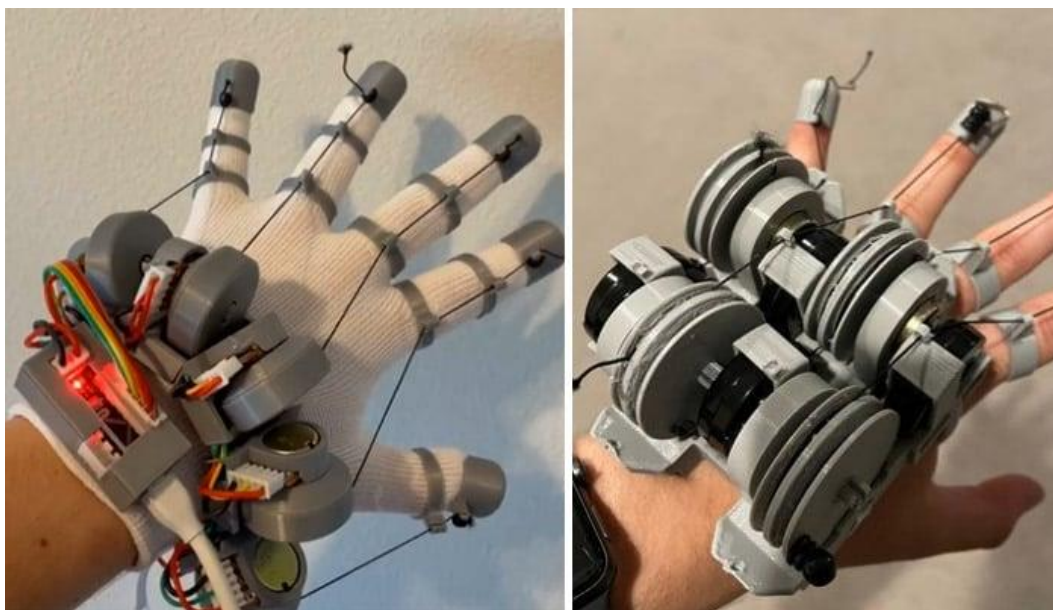
Image 3-1 LucidVR Glove Prototype3 and 4 with potentiometers (LucidVR, Lucidglove, n.d.)
