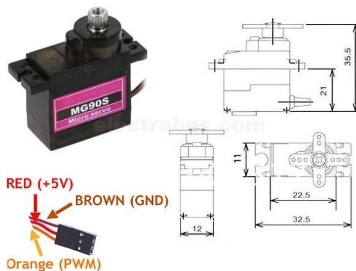
Image 4-2 Servo Motor MG90S with pinout and dimensions (Scaldas)
