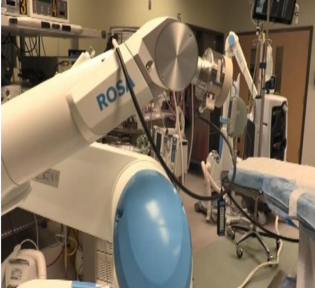
Figure 3.19 The Force-Torque Sensor of the ROSA ® Knee system (right image) attached on the Robotic Arm (left image) [83].
