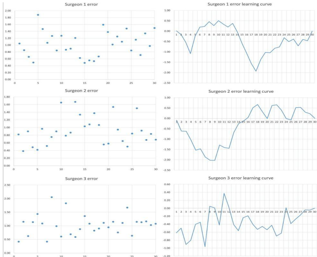
Figure 3.49 Overview of the learning curves for bone cutting accuracy among three surgeons using robot-assisted surgical system for total knee arthroplasty [98]. The Vertical Axis represents the cutting error in millimeters and the Horizontal Axis the number of operations.
