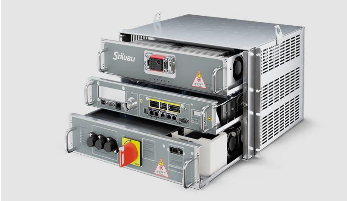
Figure 3.17 The Stäubli CS9 Robotic Arm Controller of the ROSA® Knee system [83].
