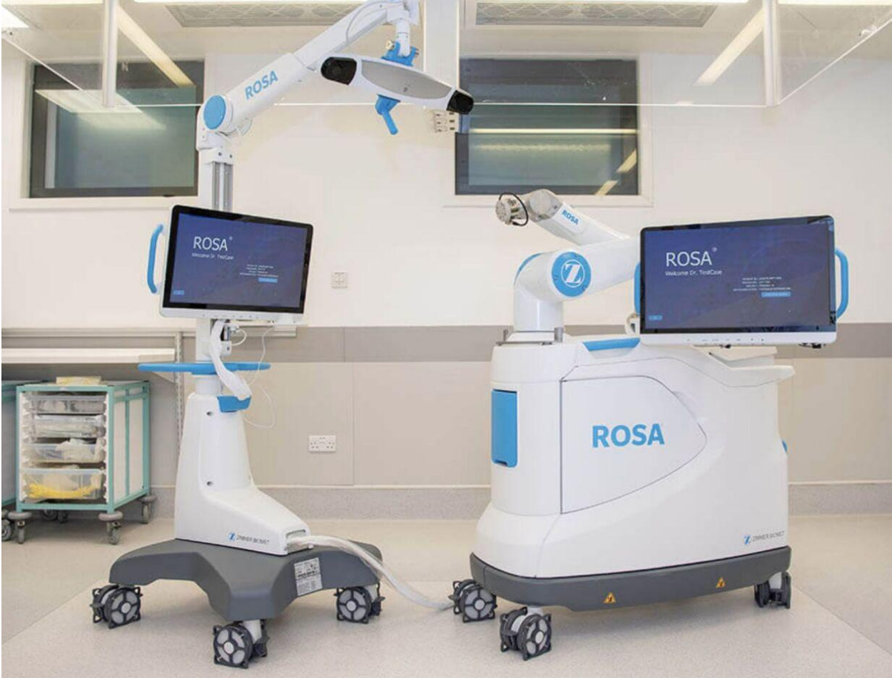
Figure 3.23 The Trolley Wheels and Steering System (in blue) of the ROSA® Knee [83].
