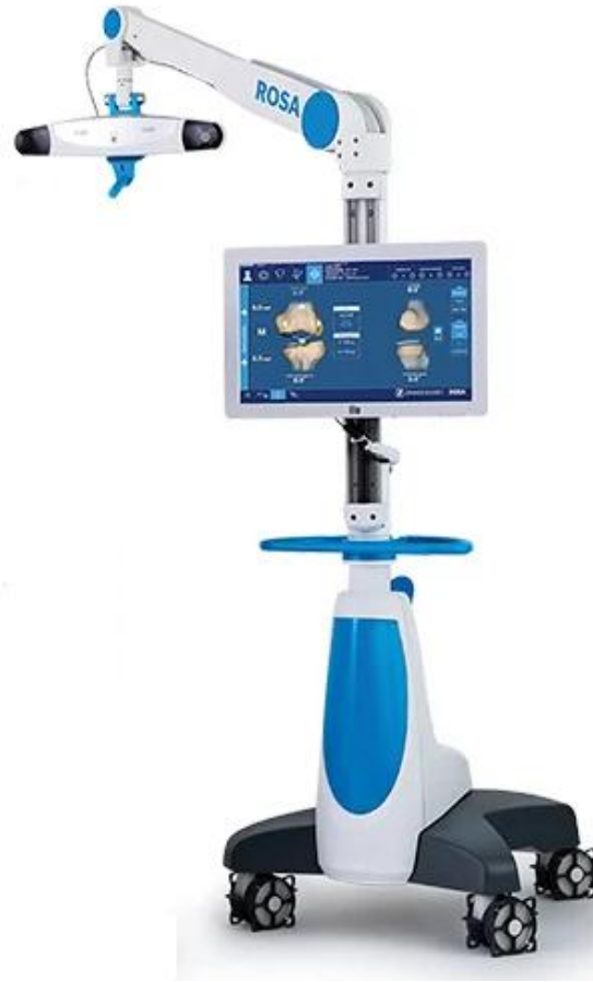
Figure 3.27 The Trolley Wheels and Steering System of the ROSA® Camera Stand (in blue) [83].
