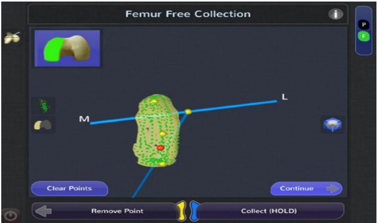
Figure 3.38 Registration of femur anatomy using the NAVIO system with the infrared probe and foot pedal for data collection [94].
