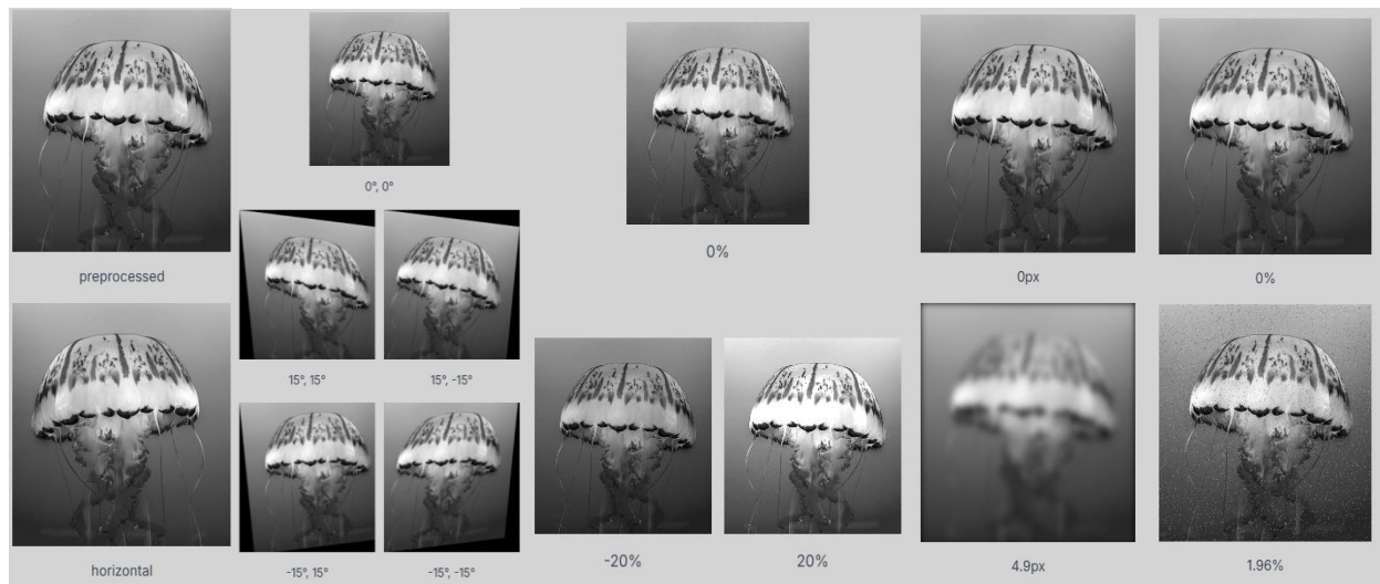
Figure 2.5 Types of augmentation techniques, from left to right Horizontal Flip, Rotation \pm 15^\circ , Brightness \pm 20\% , Blur, Noise
