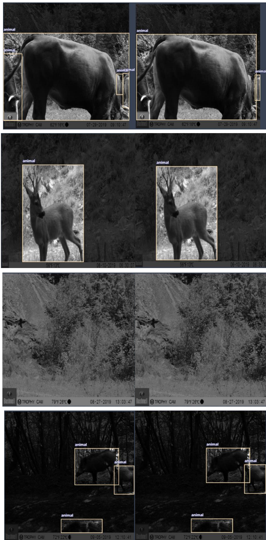
Figure 3.13 Sample of the test images, Ground Truth (left) and Model Predictions (right)
