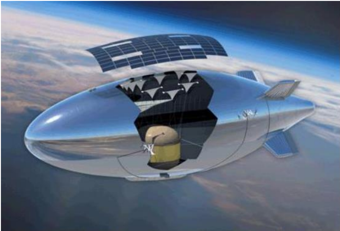
ISIS airship exploded view showing the location of the ASEA radar within the hull, and the solar photovoltaic array on the top of the hull. Source, both graphics: Lockheed Martin
