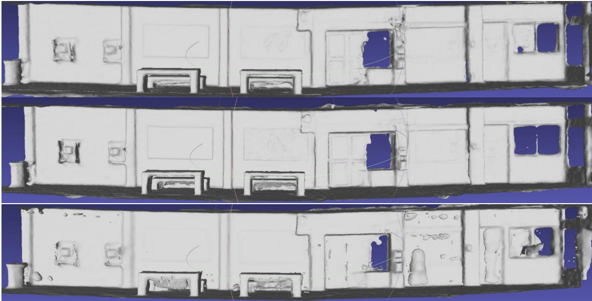
Figure 95: 3D reconstruction results for Neus-Facto (top), MonoSDF (middle), and UniSurf (bottom) with pipeline. model. sensor-depth-l1-loss-mult set to 0.8
