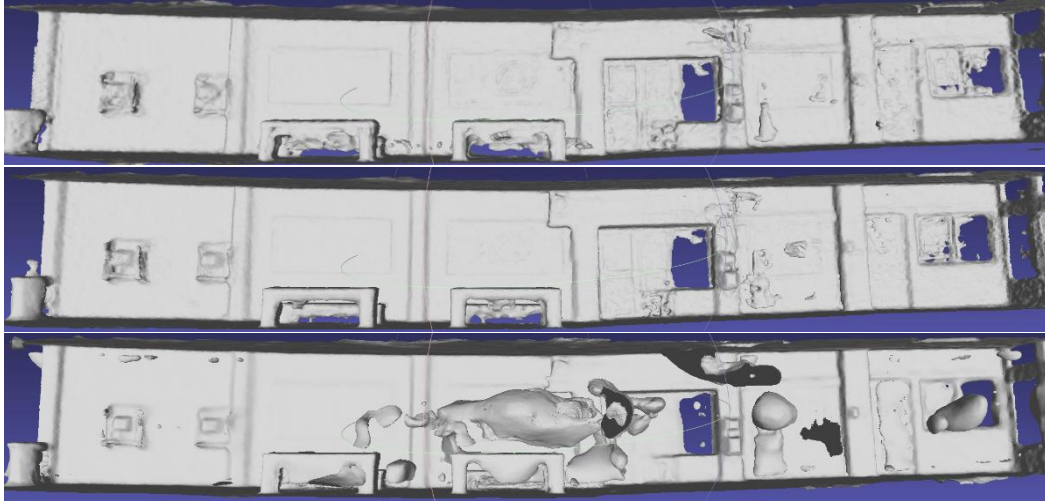
Figure 89: 3D reconstruction results for Neus-Facto (top), MonoSDF (middle), and UniSurf (bottom) with pipeline.model.sdf-field.bias set to 0.05
