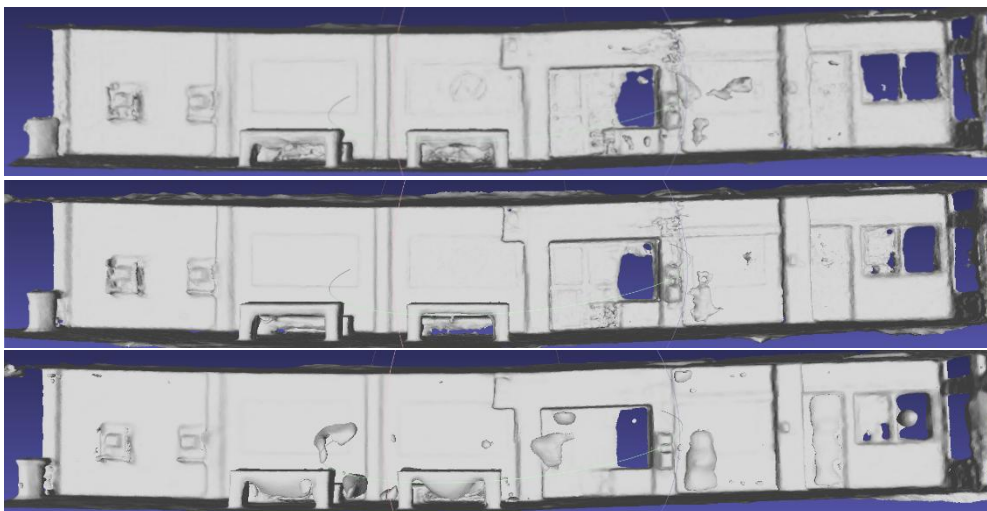
Figure 75: 3D reconstruction results for Neus-Facto (top), MonoSDF (middle), and UniSurf (bottom) using suggested parameter values.
