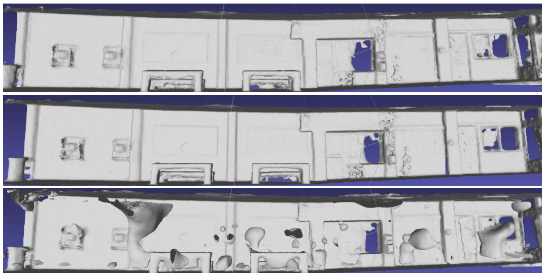
Figure 87: 3D reconstruction results for Neus-Facto (top), MonoSDF (middle), and UniSurf (bottom) with pipeline.model.sdf-field.geometric-init set to False
