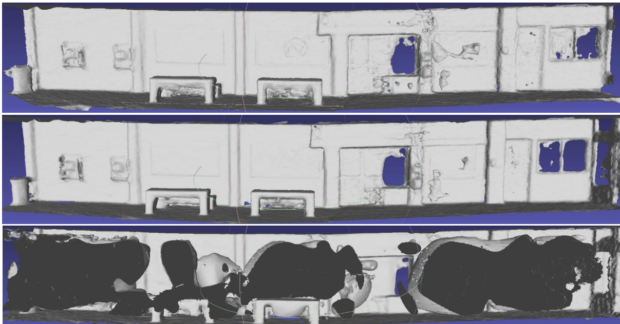
Figure 97: 3D reconstruction results for Neus-Facto (top), MonoSDF (middle), and UniSurf (bottom) with pipeline.model.sensor-depth-freespace-loss-mult 0
