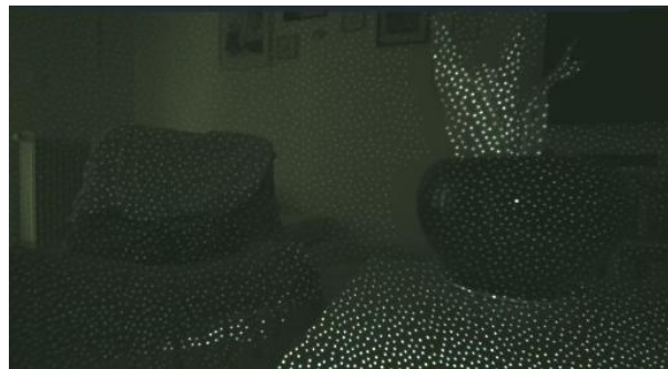
Figure 17: D455 infrared pattern
