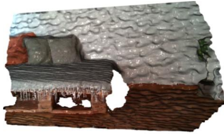
Figure 24: Colored point cloud from depth and rgb frames
