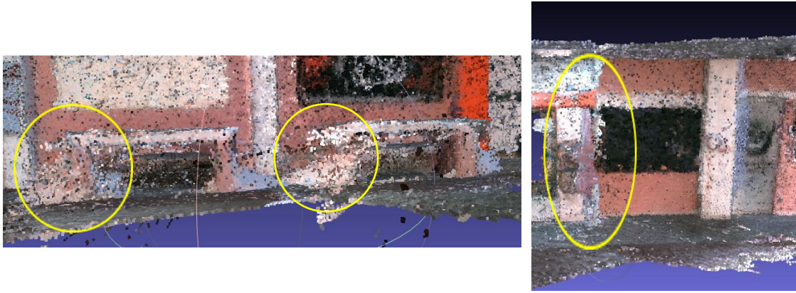
Figure 68: Misalignment or noisy areas of the final combined point cloud
