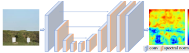
Figure 3.12. U-Net discriminator of Real-ESRGAN with spectral normalization for training dynamics stabilization. This component is crucial since the complicated degradation space imposes instabilities during training [11].
