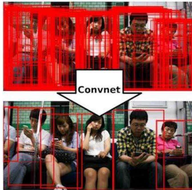
Figure 1: We propose a non-maximum suppression convnet that will re-score all raw detections (top). Our network is trained end-to-end to learn to generate exactly one high scoring detection per object (bottom, example result).
