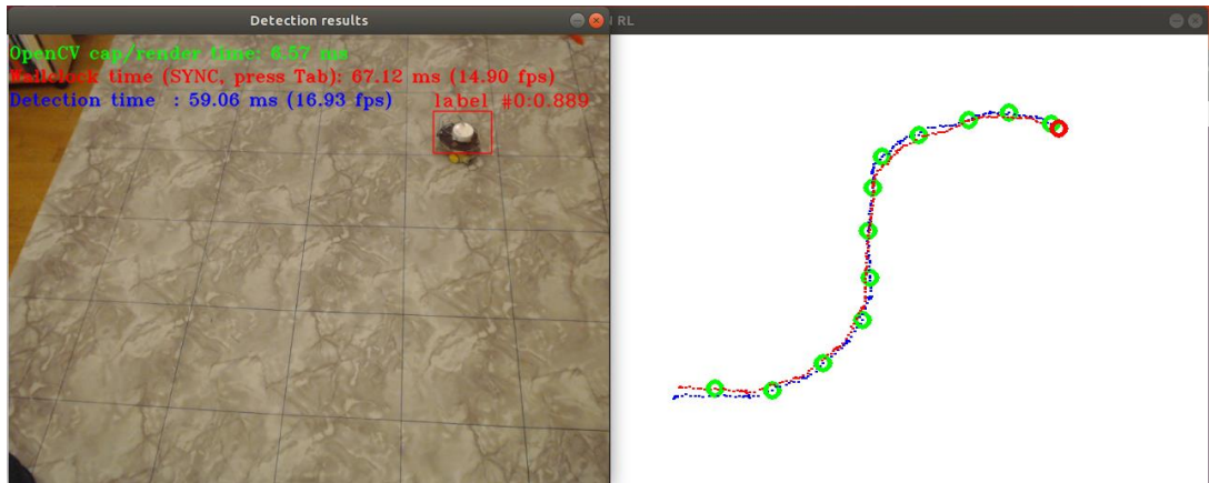
Figure 30: The camera is tilted relatively to its axis and moved at the side of the running plane. Right is the real time monitor, the red circle is the target and the green dots are the waypoints.
