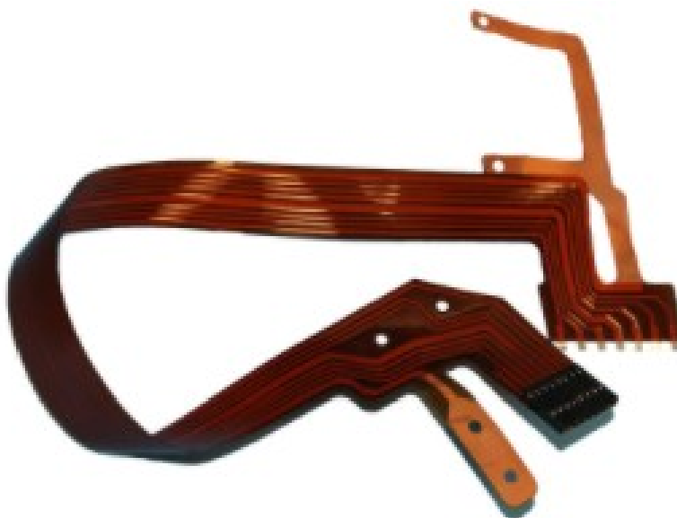
Εικόνα 4.8 Double Side flex Πηγή : Flexible Printed Circuits | Solution to Electronic Packaging Needs (allflexinc.com)
