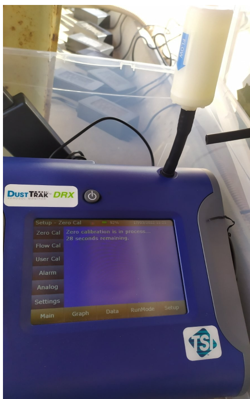
Illustration 53: Step two for zeroing of TSI.
